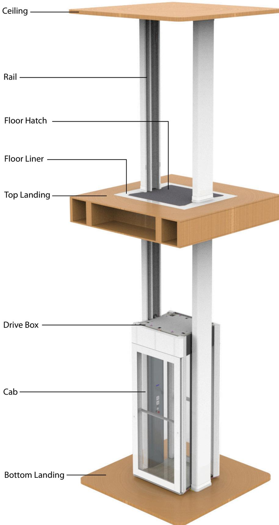
Figure 1: Luma lift diagram
