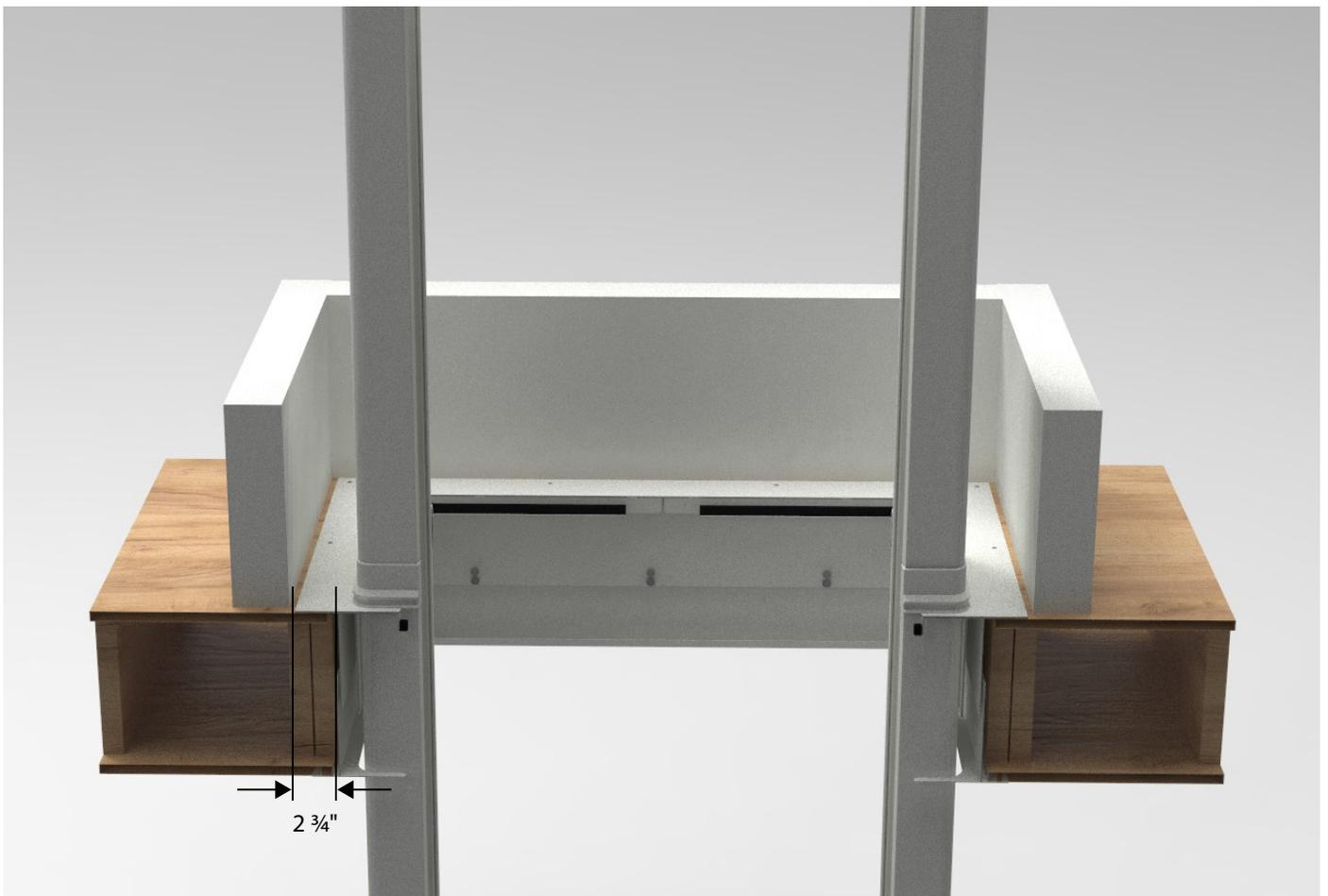
Figure 18: Minimal Clearance From Wall To Floor Opening
