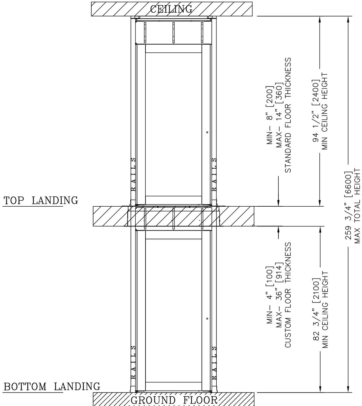
Figure 19: Elevation View - 2000 mm (78 3/4") Cab
