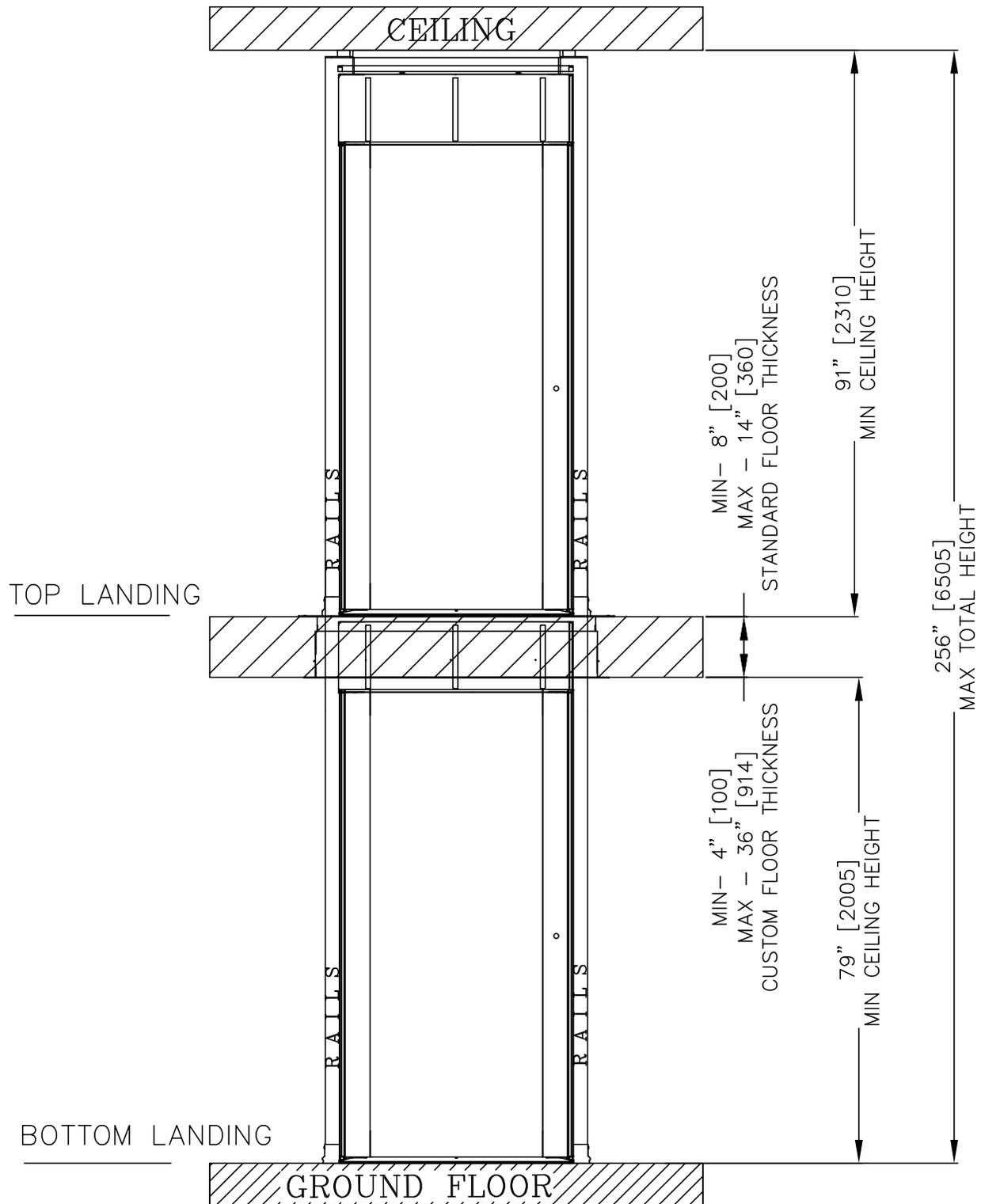
Figure 20: Elevation View - 1905 mm (75") Cab
